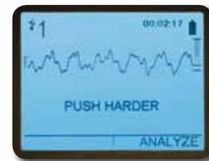
If your CPR chest compressions are too shallow, you will be prompted to "Push Harder."
